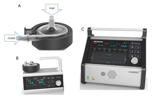
Figure 1 The OASSIST<sup>®</sup> ECMO system of the Jiangsu STMed Medical Technology Co. Ltd.. (A) The centrifugal pump and the driver base; (B) the driver used for driving the rotation of the centrifugal pump; (C) the main control unit used for monitoring relevant parameters.
