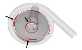
**Figure 9** Distribution of areas with 3D shear stress >150 Pa at 4,000 rpm and 5 L/min.
