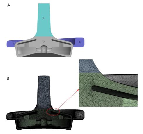
**Figure 4** Fluid model and Meshing. (A) The model used for calculation, including two static zones (a and c are the static zones) and a rotation zone (b is the rotation zone). (B) Grid partitioning. The boundary layer was added to the solid wall surface, and denser grids were used in the rotor zone.
