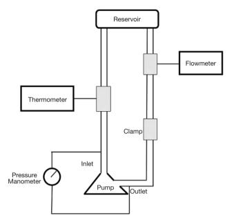
Figure 3 Test loop.
