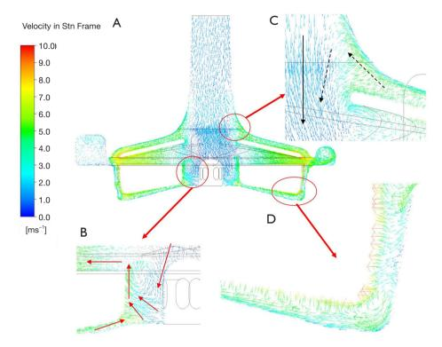
**Figure 8** Velocity vector distribution at 4,100 rpm and 8 L/min: (A) inlet midline section; (B) velocity vector distribution in the midline section near the bottom support of the rotor; (C) velocity vector distribution in the gap between the top case of the blade and the volute; (D) velocity vector distribution in the midline section of the gap between the rotor bottom and the volute.
