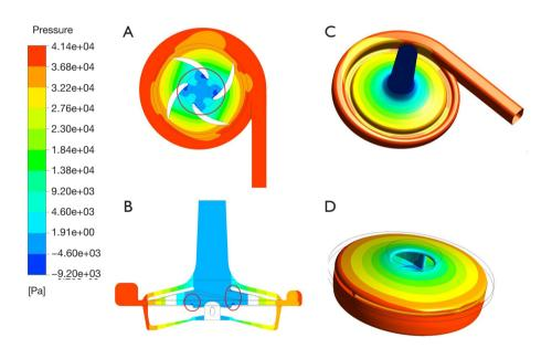
Figure 6 Distribution of static pressure at 4,100 rpm and 8 L/min: (A) blade middle section; (B) inlet midline section; (C) inner surface of the whole apparatus; (D) impeller/rotor surface.
