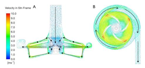
**Figure 7** Velocity vector distribution at 4,100 rpm and 8 L/min: (A) velocity vector distribution in the midline section of the pump inlet; (B) velocity vector distribution in the horizontal section in the middle of the rotor blade of the pump.
