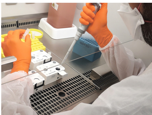
Figure S1 Sample loading into the Idylla cartridge under a BSC-2 hood.
