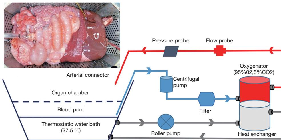
**Figure 2** The schematic of normothermic machine perfusion (NMP) device. NMP device was designed as an opened perfusion circuit with continuous (no pulsatile) arterial flow at a temperature of 37.5 °C. The device consists of three layers: from the bottom to surface are the thermostatic water box, the open blood reservoir and the organ chamber respectively. The key components are an oxygenator, heat exchanger, flow probe, pressure probe, centrifugal pump, roller pump and Connecting Pipes.
