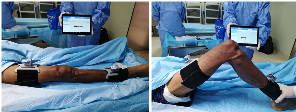
Figure 1 The goniometer for recording the range of motion in the knee joints. The 2 components are attached to the proximal thigh and the distal calf.
