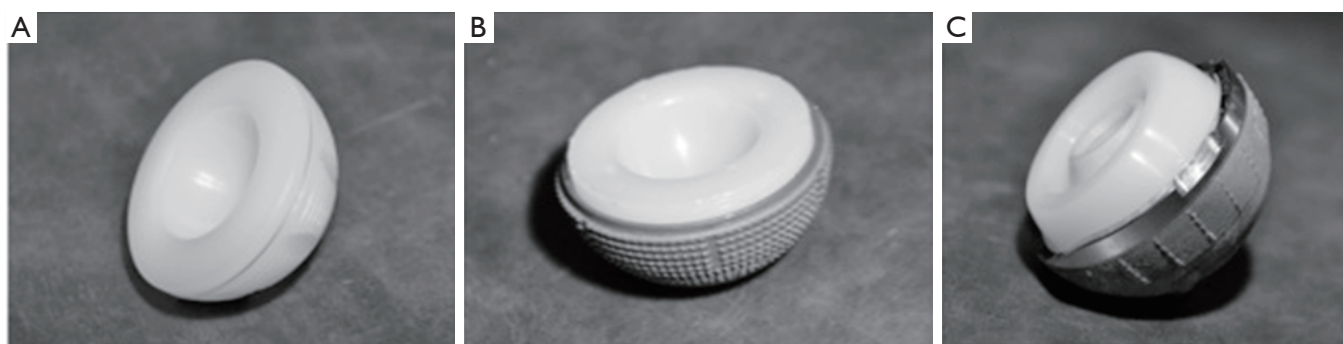
Figure 1 The three types of acetabular cup used (all manufactured by Zimmer Inc., Warsaw, IN, USA): (A) cemented Durasul® highly cross-linked all-PE cup; (B) un-cemented Allofit® metal-backed titanium acetabular cup with press-fitted Durasul® highly cross-linked PE liner; and (C) un-cemented Stafit® dual-mobility CoCr acetabular cup with mobile Sulene® conventional PE liner.
