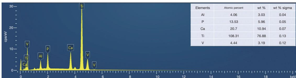
**Figure 2** Representative EDS analysis of the MAO-treated  $Ti_6Al_4V$  scaffold. EDS, energy-dispersive X-ray spectroscopy; MAO, micro-arc oxidation.
