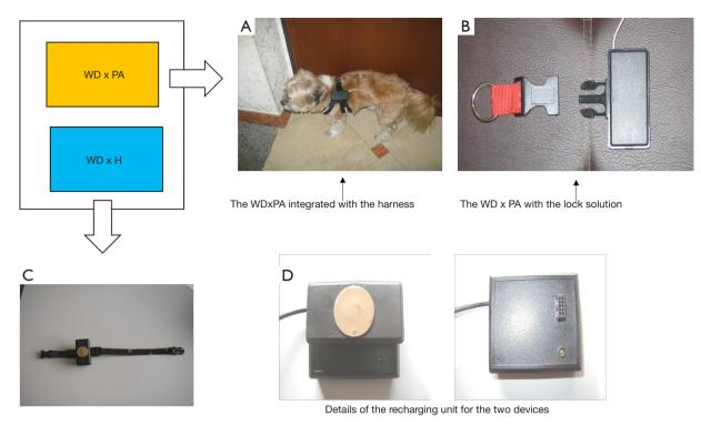
Figure 1 The components of the *wearable sensor* unit (Kit).
