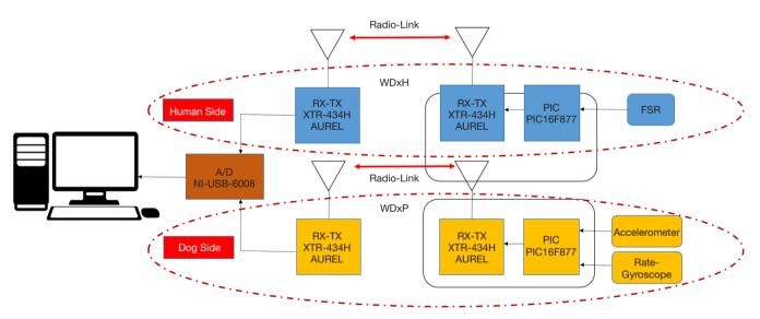
Figure 2 The architecture of the *telemetric system*.
