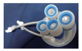
**Figure 2** Multi-hole port for single-port surgery (LapSingle Vision<sup>TM</sup>).
