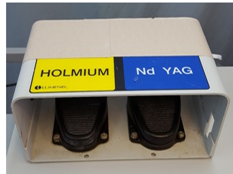
Figure 5 Dual-laser generator pedal for alternative use of Nd:YAG and Ho:YAG.
