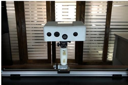
**Figure 2** The novel 3D facial scanner is installed on a sliding track and driven by a motor to move automatically. The imaging process takes less than 20 seconds. Please also see the [Video S1](#).
