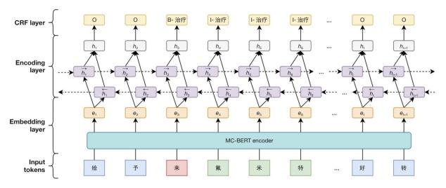
Figure 7 The model architecture of named entity recognition. CRF, conditional random field; MC, medical; BERT, bidirectional encoder representation from transformers.
