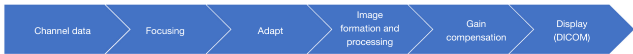
Figure 1 Image processing chain for Adapt (name of aberration correction algorithm) images. For the standard images, the Adapt and gain compensation sections were omitted. DICOM, Digital Imaging and Communications in Medicine.
