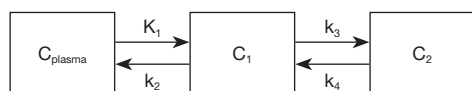
Figure 1 Diagram of the tracer kinetics of ^{68}\text{Ga} -DOTATATE. A 2-tissue compartment model is used. K_1 describes the binding to the receptor, k_2 the displacement from the receptor, k_3 the cellular internalization, and k_4 the externalization. ^{68}\text{Ga} -DOTATATE, ^{68}\text{Ga} -DOTA 0 -Tyr 3 -octreotate.
