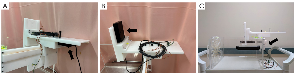
Figure 3 The motor driver with three-direction arrangement. (A) The arrangement in X-direction. (B) The arrangement in Y-direction. (C) The arrangement in Z-direction. The black arrows pointed out the different position of the motor driver, which could deliver the water phantom in one-direction movement.
