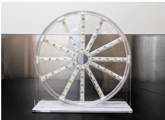
Figure 4 The structure of distortion phantom.
