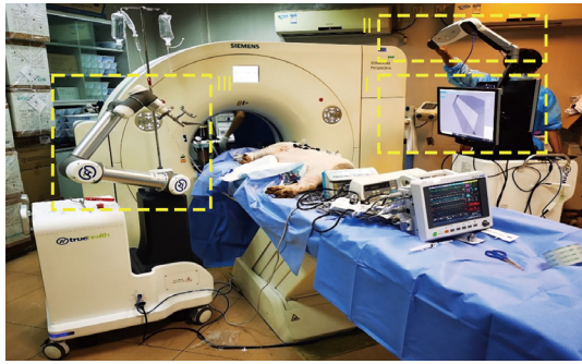
Figure 1 Robot-assisted navigation system in surgery. (I) The surgical planning system. (II) The photoelectric navigation system. (III) The robotic arm positioning and puncture system.
