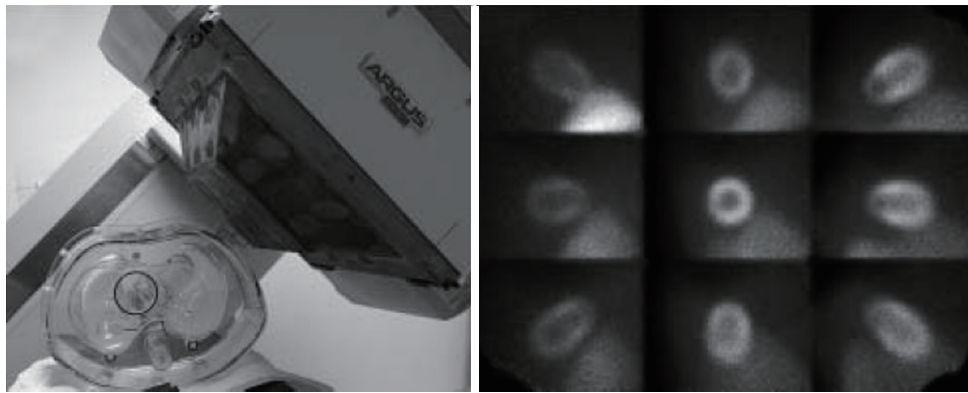
Figure 11 Left: experimental setup of the 9-pinhole MPI SPECT system with a torso phantom. Right: non-multiplexed projection data of the phantom with cardiac and liver uptakes [courtesy of Funk et al. (64)].
