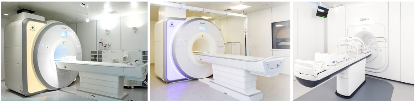
Figure 1 The three types of MRI scanners. Left: a normal 1.5 T diagnostic MRI scanner. Middle: a 1.5 T MRI-simulator. An anterior coil and its coil frame, as well as knee rest and ankle stock are shown. An external 3-dimensional laser is equipped. Right: a 1.5 T high field integrated MR-LINAC. There is neither in-bore nor external laser equipped with the MR-LINAC. MR-LINAC, MRI and linear accelerator system.
