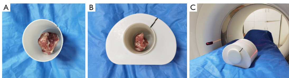
Figure 2 Assembly of the 3D-printed phantom. (A) The specimen placed into the insert. (B) The phantom assembly. (C) CT scanning of the 3D printed phantom. 3D, three-dimension; CT, computed tomography.
