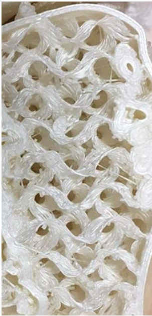
Figure 11 An example of a 3D print with an infill of 20% with gyroid structure, resembling the tactile feel of cancellous bone.
