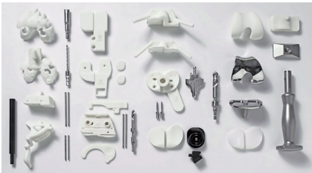
Figure 1 ConforMIS' iTotal joint replacement kit includes a set of various surgical tools required for the knee replacement surgery mainly. Most of them are printed using 3D SLS printer. Source: https://3dprint.com/78272/conformis-3d-printed-knee/ . SLS, selective laser sintering.
