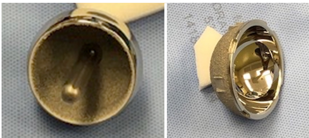
Figure 4 Zimmer Biomet uncemented recap femoral and Magnum acetabular components. Cobalt chrome as cast implants fully porous coated with titanium alloy plasma spray. Additional hydroxyapatite coating on femoral implant.
