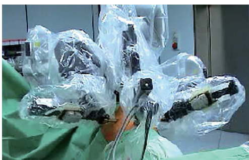
Figure 1 DaVinci Standard System, provided only with 3 arms.
