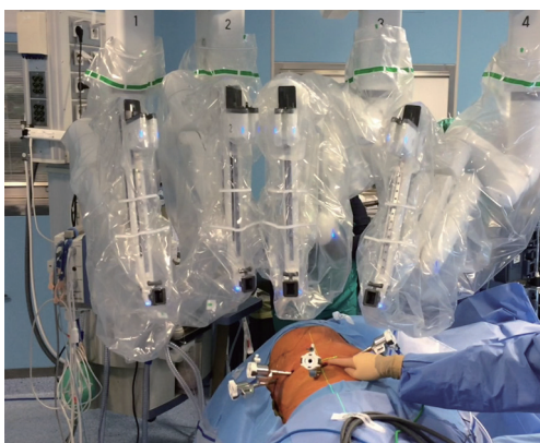
Figure 2 Docking phase of Xi System, assisted by laser targeting system.
