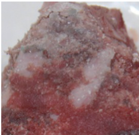
Figure 8 Transverse cut showing morphology of bone-cement bonding in a typical augmented vertebral body.
