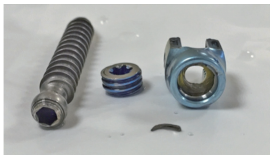
Figure 6 Pictures of the dislocated polyaxial screw and the securing nut.
