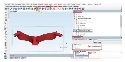
Figure 9 The new object of target posterior surface was created and "Offset" function will be used to generate the navigation template.
