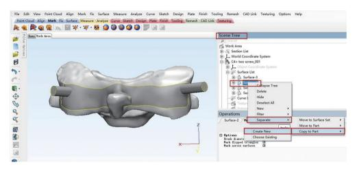
Figure 8 The target posterior surface was separated to create new object.
