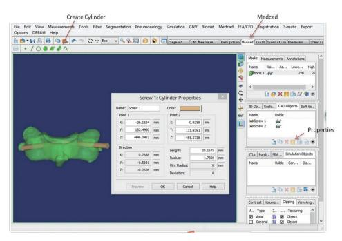
Figure 4 Cylinders were created to simulate the C4 pedicle screw trajectory.
