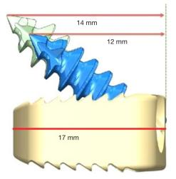
Figure 1 Image showing standalone cage with the size of screws and length of the implant.
