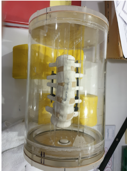
Figure 3. Experimental construct of lumbar spine model instrumented with titanium pedicle screws. 4 pedicle screws (CarboClear™, CarboFix Orthopedics, Herziliya, IL, USA) were inserted into the left pedicles and 2 pedicle screws were inserted into the right pedicles, and connected by 2 longitudinal rods. The model was suspended on plastic rods and immersed in water.
