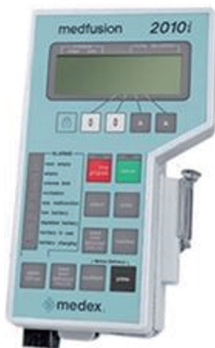
Figure 5 Medfusion 2010i infusion pump.
