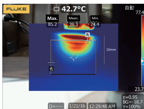
Figure 2 Preliminary experiment on chicken muscle tissue to measure the temperature. A cone-shaped high temperature lesion was observed. The maximum temperature was raised to 97.9±2.1 °C.
