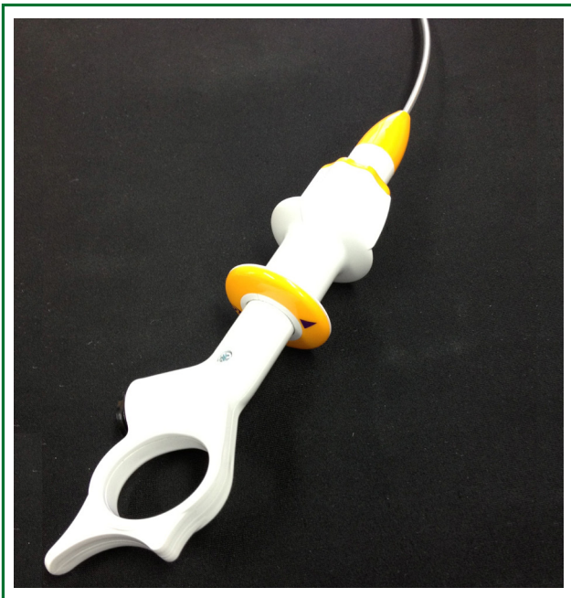
Figure 1. SuperDimension steering catheter handle: note the black arrows on the yellow ring of the catheter neck indicating the turning direction of the locatable guide.
