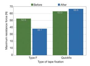
**Figure 10** Maximum resistance force [Newton (N)] under skin coating agent under skin coating agent using a 24-Fr tube. Quickfix did not show an obvious change, although the maximum resistance force type F decreased.
