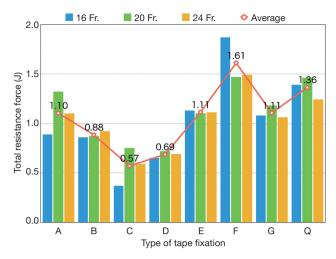
**Figure 7** Average values of total resistance force [Joule (J)] under each tube size condition. The data showed that the resistance was the highest for type F followed by Quickfix.
