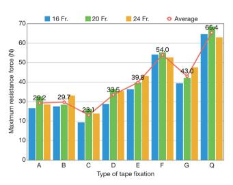
**Figure 8** Average values of maximum resistance force [Newton (N)] under each tube size condition. The data showed that the resistance of Quickfix was the highest followed by type F.
