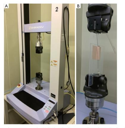
**Figure 5** Tape fixing strength test. (A) Autograph AGS-X (Shimadzu Corporation, Kyoto, Japan). (B) The tube pulling out in the long axis direction at a speed of 1,000 mm/min. During pulling it out, the maximum resistance force (Newton) and total resistance force (Joule) were measured as fixing strength by Autograph AGS-X.
