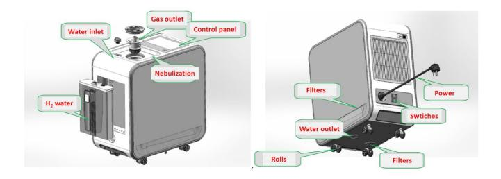
**Figure E1. A schematic diagram of the Hydrogen/Oxygen Generator (model AMS-H-03).** Courtesy of Shanghai Asclepius Meditec Co., Ltd. (Shanghai, China).
