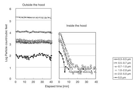
Figure 2 Concentration of airborne particles with size greater than 0.3  $\mu$ m, inside and outside the positive-pressure hood with the FFU switched on with airflow rate 0.19 m<sup>3</sup>/min. Saline was atomized outside the hood and airborne particle concentrations of the air inside and outside the hood were measured at several time intervals after the atomization.
