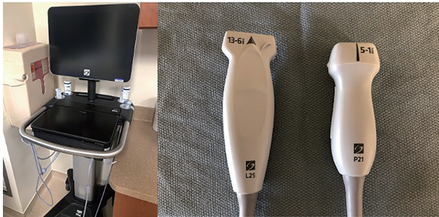
Figure 4 Point of Care SonoSite Ultrasound on top. Two probes visible below, with a high frequency linear transducer on the left and a small footprint phased array transducer on the right.
