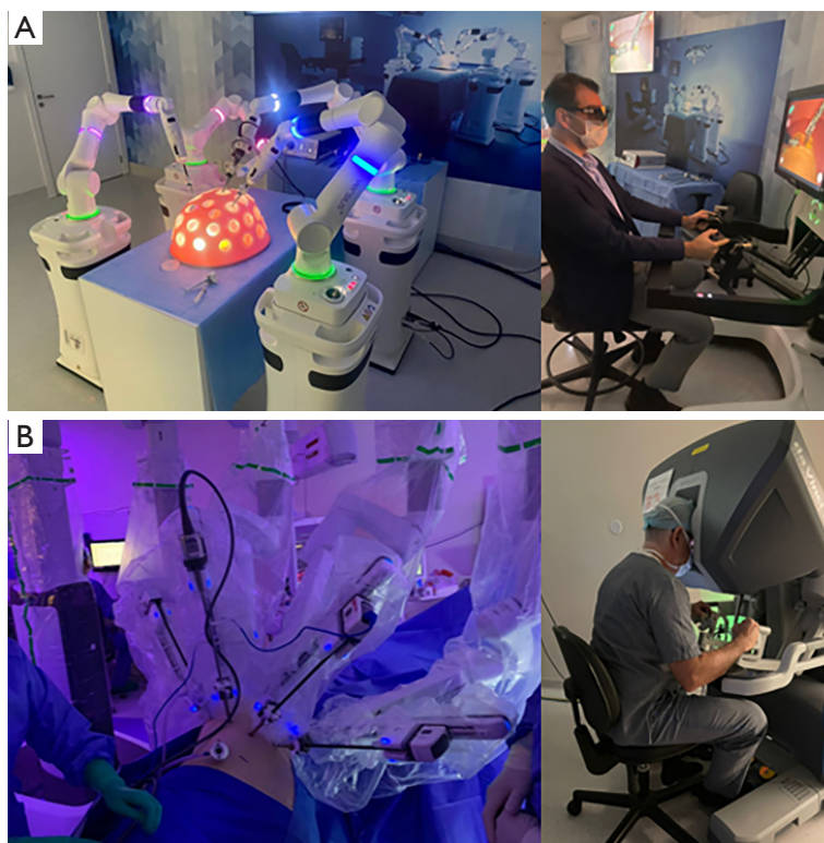
Figure 4 The two most disseminated platforms. (A) Versius (CMR Surgical) with its modular arms disposition, 3D monitor, joysticks, and 3D glasses; (B) da Vinci (Intuitive) in its Xi model with four-arms connected by a single tower and the surgeon immersed in the console.
