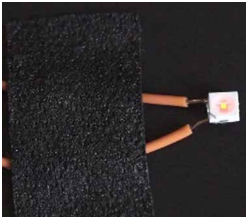
Figure 7 The voltage output of piezoelectric nanogenerator at the natural condition (closed chest) can make LED light continue to shine. LED, light emitting diode.
