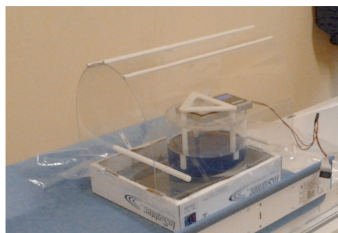
Figure 3 Weighing system with shield and external commando.
