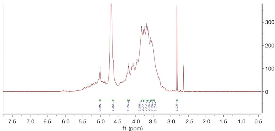
**Figure 1** The  $^1\text{H}$ -NMR spectra of poly-GTAC- $\beta$ -CD.
