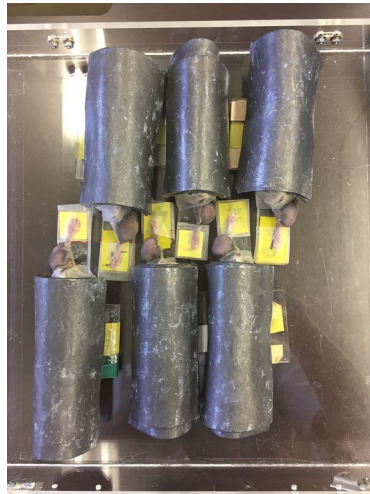
Figure S1 The device to fix mice for irradiation. During irradiation, the head, trunk, and left leg of mice are shielded by lead plates, while the tumor-bearing right leg fixed with adhesive tapes is not shielded. Although the mice are different from those used in this study, the same device was used.
