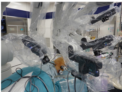
Figure 3 The picture of robotic arms of hinotori consisting of eight axes that enable more flexible movement and prevent them from interfering with each other. Software-based calibration of the trocar position without docking an arm with a trocar provides a sufficient space in a clean field and protects collisions among arms outside the body.
