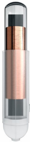
Figure 9 LOCALizer™ RFID breast marker which comes with a unique number for each tag (Hologic Inc., Marlborough, MA, USA).
