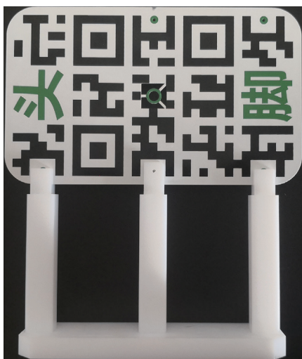
Figure 3 Positioning QR code. A board with a printed QR code, together with green head/feet direction indication letters (in Chinese). This board will be placed beside the operating area before navigation start. QR code, quick response code.
