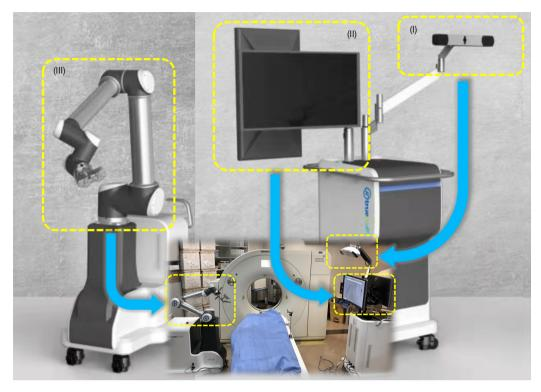
Figure 1 The robotic-assisted navigation system. (I) The photoelectric navigation system used to track the position of the robotic arm and the patient; (II) the surgical planning system employed for the precise planning of the needle insertion path; (III) the robotic arm positioning and puncture system responsible for accurate positioning of the needle holder and assisting with needle insertion.
