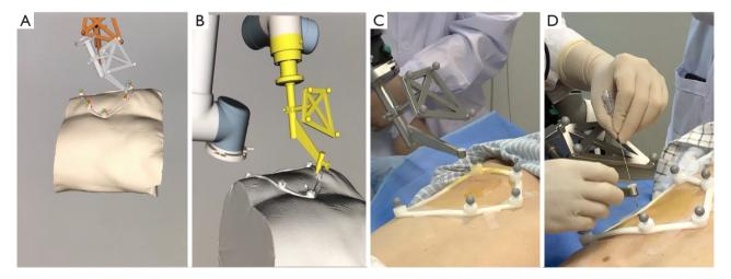
**Figure 3** Navigation planning and robotic-assisted positioning puncture process. (A) Registration of the 3D model to the patient's precise position; (B) motion planning and simulation of the robotic arm to ensure avoidance of any obstructions during the procedure; (C) precise positioning of the needle holder. The robotic arm automatically positions the needle holder in alignment with the planned trajectory; (D) needle insertion guided by the robotic-assisted system. 3D, three-dimensional.
