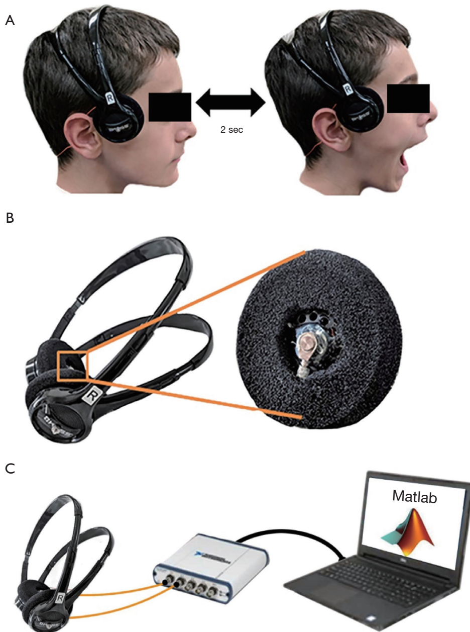
Figure 1 Recording setup used for capturing TMJ AEs. (A) Each subject wore the headset and performed 10 repetitions of opening and closing their mouths, at a rate of 1 cycle per 4 seconds while watching an animation to help maintain consistent speed and movement. (B) AEs were recorded from both TMJs simultaneously while performing the exercises using uniaxial accelerometers embedded into a headset form-factor for convenient placement superficial to the TMJ. (C) The headset accelerometer signals were captured with an NI-DAQ system using a software program written in Matlab. TMJ, temporomandibular joint; AE, acoustic emission.
