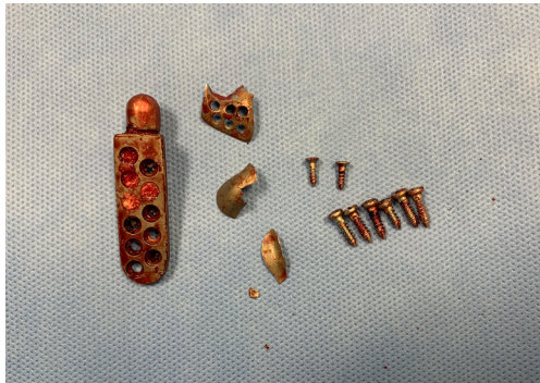
Figure 5 Same device following removal demonstrating fractured fossa component.
