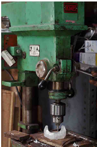
Figure 1 Pillar drilling machine used to maintain parallelism.
