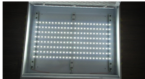
Figure 3 An array of low-power LED lamps.
