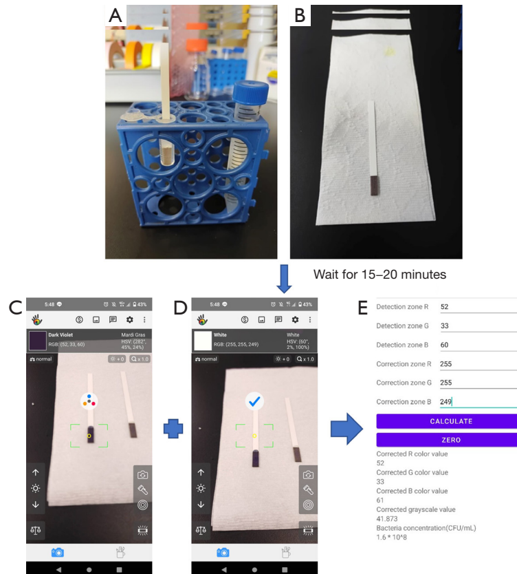
Figure 5 User procedure. (A) Dipping our test strip into the sample; (B) test strip placed at room temperature and allowed to dry for 15–20 minutes; (C) color grab used to obtain RGB value from the detection area of the test strip; (D) obtained RGB value of the white area above the test strip used as the calibration standard; (E) input of the RGB value from the detection area in (C) and the white area in (D) into the APP for calculation. CFU, colony-forming unit; APP, application.
