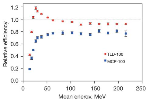
**Figure 3** The relative efficiency of the TLD-100 and MCP-100. Dash line is relative to 6 MV photon beam. Red points is the relative efficiency of proton dose calibration for TLD-100. Blue points is the relative efficiency of proton dose calibration for MCP-100. TLD, thermoluminescent dosimeter.
