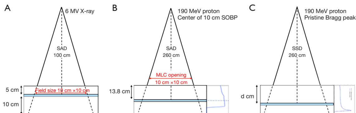
**Figure 1** Set-up diagram of dose calibration and validation for photon and proton. (A) 6 MV X-ray dose calibration and validation; (B) proton dose calibration; (C) proton dose validation at different depths. d, depth; SOBP, spread-out Bragg peak; SAD, source-to-axis distance; SSD, source-to-surface distance; MLC, multileaf collimator.
