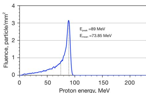
**Figure 5** Proton energy spectrum at the dose calibration condition, which is dominated by 89 MeV and has mean energy of 73.85 MeV.
