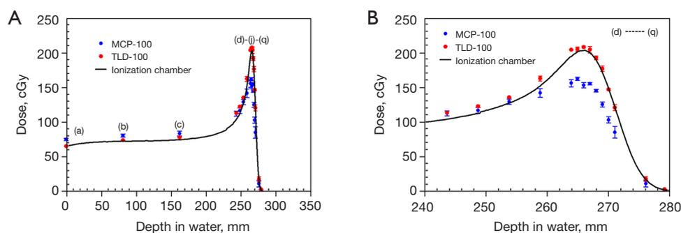
**Figure 2** The comparison results of proton dose measurement between ionization chamber and TLDs. (A) The Bragg peak of 230 MeV; (B) part of 230 MeV Bragg peak from depths of 24 to 28 cm. (a) 0 mm; (b) 80.8 mm; (c) 161.6 mm; (d) 242.4 mm; (j) 264.6 mm; (q) 277.8 mm. TLDs, thermoluminescent dosimeters.
