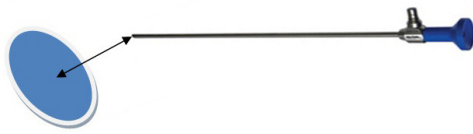
Figure 6 For the same surgical field, a clear image can be acquired using a fixed focal length and maintaining a specific distance between the target and the lens.
